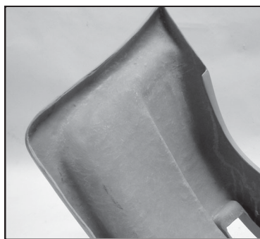
PHOTO 20 Mat only construction. Note the puddle of resin pooled into this low spot on this part made only with chopped strand mat
