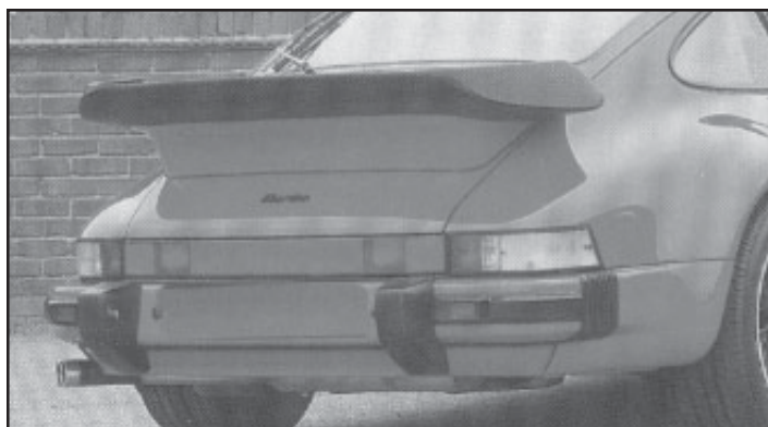
PHOTO 16 Rear Bumper Blade The aluminum bumper blade on the back of the 74-83 911 SC's weighs over 20lbs.
