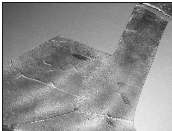
PHOTO 21 Cloth mosaic. Here is a very strange example of a lower spoiler which was laminated with dozens of tiny square pieces of light weight cloth. I can only imagine that this was the work of a really poor laminator who couldn't manipulate material that was more than a few inches square. Note fracture. This part wasn't even strong enough to survive shipping.
