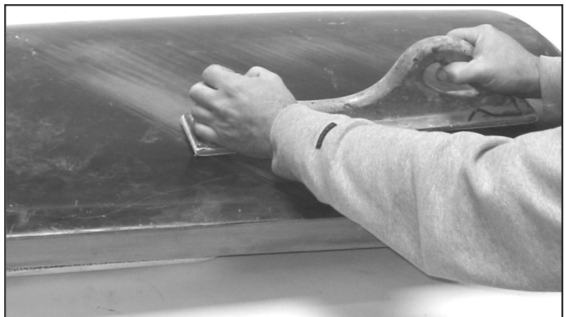
PHOTO 7 Block sanding a door Using a long board file to hand sand a door to remove dents and waves
