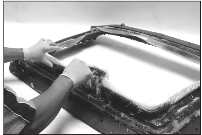
PHOTO 4 Hand laminating a Decklid Liner In this photo the laminator is "wetting out" mat and cloth. Forming it to the contours of the liner mold section.
