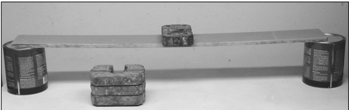
PHOTO 23 Particle board demonstration. Notice how far this common piece of 5/8 inch particle board sags under only 10lbs.
