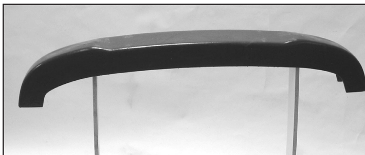
PHOTO 17 Bumper blade on stand The bumper blade has been mounted on a stand to make it easier to work on.
