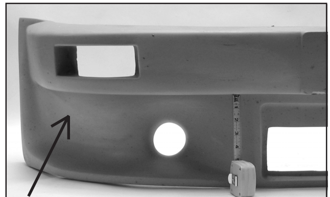
PHOTO 5 Example of a poorly made bumper. Notice how the top edge of this bumper is severely warped. This is an example of part that should be returned as unsatisfactory. The amount of time and energy needed to repair the warping exceeds the initial cost.
